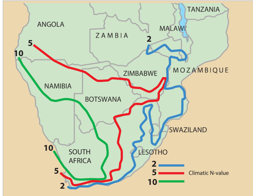
Figure 5.5 - Climatic N-value map of southern Africa 7 (currently does not cover the entire SADC region)
