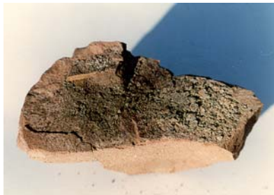
Sample of weathered, decomposed basalt, showing altered clay minerals in rock vesicles and cavities.
