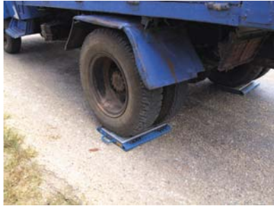
Measurement of rear axle load using portable weighbridge.
