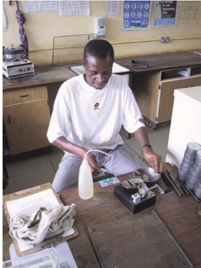
Liquid Limit device used in the determination of the plasticity index of a soil.
