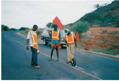
Visual condition survey.
