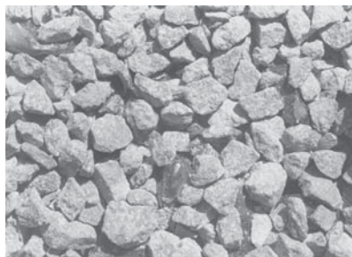
Cubical chipings are essential for good particle interlock in Chip seals.
