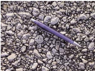
Example of a 10 year old crushed coral stone surfacing aggregate which does not meet traditional strength and durability criteria but, nonetheless, has performed very satisfactorily in a LVSR situation.
