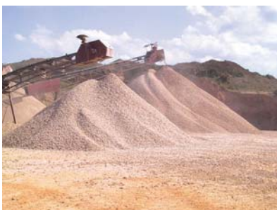
Crushed limestone is a typical “standard” material that is produced by crushing of blasted, massive rock to a specified grading.
