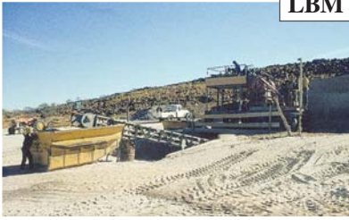
A small, simple crushing/ screening plant can be combined with labour-adapted tractor operations.
