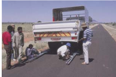
Measuring bearing capacity using Benkelman Beams.
