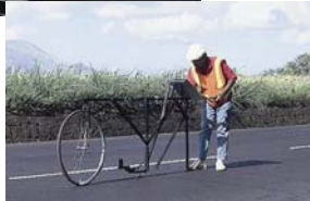
Roughness can be measured by using rapid or slow measuring devices such as a Bump Integrator or Merlin device.
