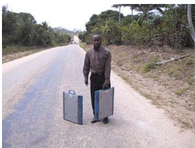
Portable weighbridge system.
