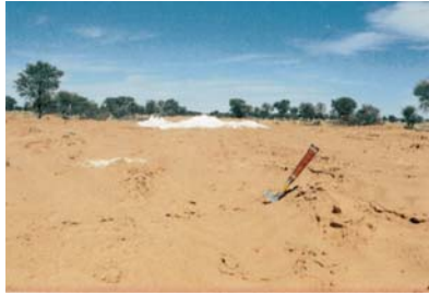
When mixed in the appropriate proportion, two non-standard materials, such as Kalahari sand and Calcrete, often satisfy the specifications of a standard/traditional material.
