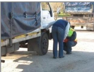
Re-checking the front tyre manufacturer's rating. The operator and traffic officer assist each other with the collection of data to eliminate errors.
