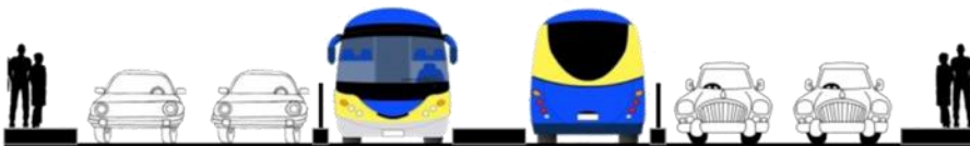
Dedicated lanes for bus rapid transit
