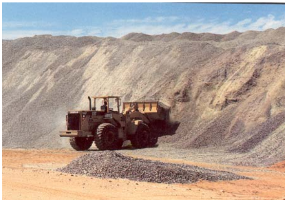
Crushed limestone—a traditional, processed materials typically specified for the base layer of LVRs. Is this relatively costly material type necessary? NO!
