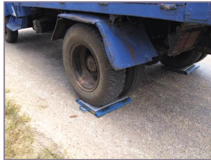
Measurement of rear axle using portable weighbridge
