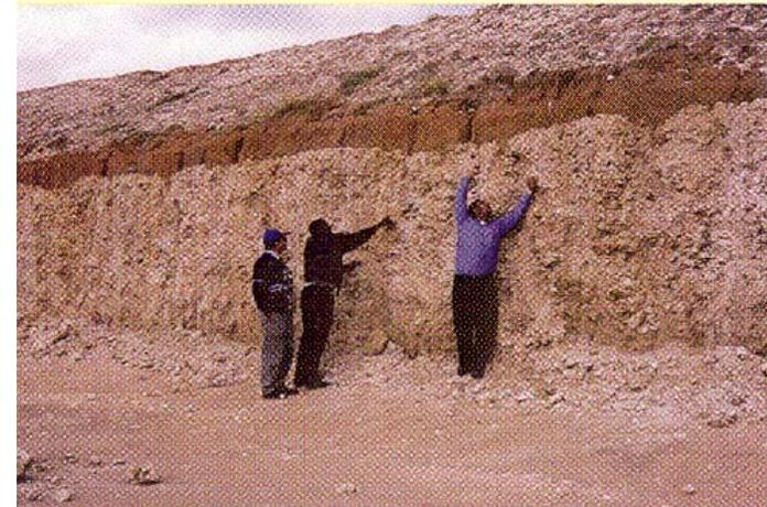
*Traditional specifications for base gravels typically specify a soaked CBR @ 98% MAASHO of 80%, PI of <6 and adherence to a tight grading envelope. However, research in the region has shown that when due consideration is given to factors such as traffic, subgrade strength, drainage, pavement cross-section, etc, substantial relaxations can be made on selection criteria with significant cost savings*
