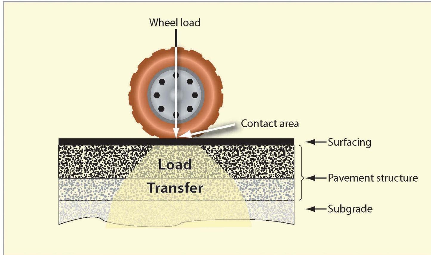
Spread of wheel load through pavement structure
